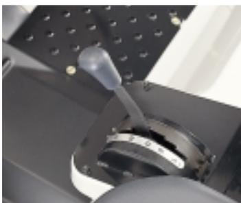
**Automatic Transmission:** The resin shift lever knob is large and textured for easy operability. The automatic transmission shifts from L to 2 to D, even when set in the D range (02-, 42- Model).
